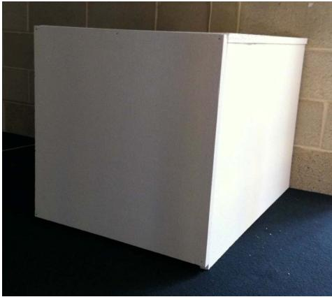
**Figure 2. Blank Waldo (600x600x900mm) in the shape of a kitchen appliance that was constructed with white polystyrene foam.**
