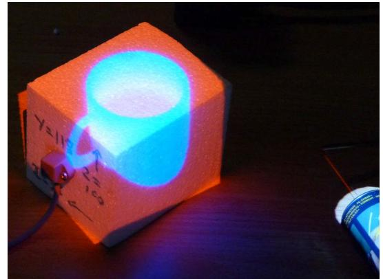
**Figure 1. Creating a physical mug from a square block of foam using Augmented Foam Sculpting**
